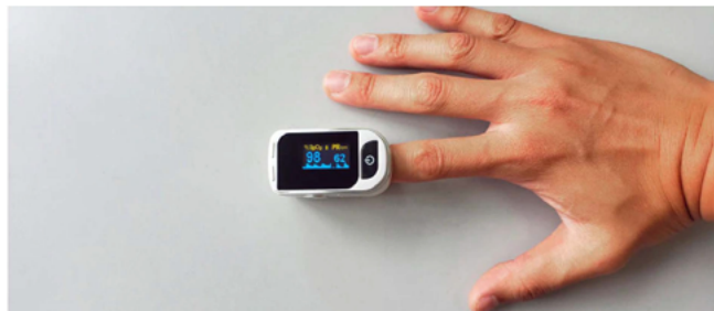
Figure 11: An example of a pulse oximeter
